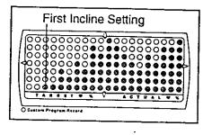
matrix will be dark. The first incline setting of the program will be shown in the third column (see the drawing above); the next seventeen incline settings are shown in the seventeen columns to the right.
